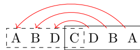
Figure 9.44: Here we see the Z box representation of the algorithm. The solid box is our current Z box, and the dashed box is the duplicate of the Z box, but reversed from the start of the current Z box. The red arrows indicate where we lookup to start evaluation of this index.
